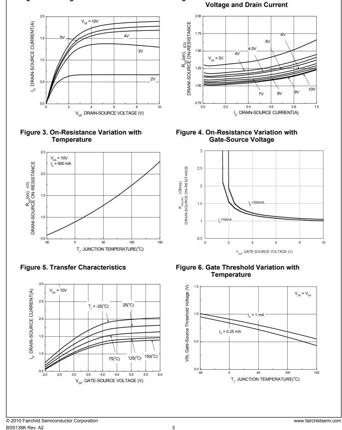
Figure 2. On-Resistance Variation with Gate
